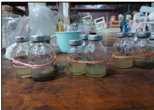
Figure 2: Anaerobic Microcosm of aquifer sediments exhibiting growth post incubation
